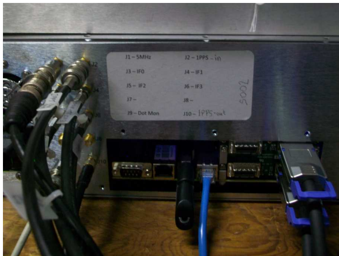
Figure 6: A closeup of the back of the RDDBE-S unit showing the connections.
