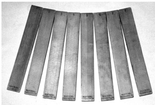
Tone Bars. These wooden tone bars give the whole notes in an octave when they are dropped, one by one, onto a hard floor. Unlike the bars of a xylophone, these all have the same length, but have different thicknesses, with the thinner bars having the higher frequencies. When they are dropped, they flex transversely, with the nodes 22.4% of the way in from the ends. This set was made by Max Kohl of Chemnitz, Germany, and is in the Greenslade Collection. (Photograph and Notes by Thomas B. Greenslade, Jr., Kenyon College)
