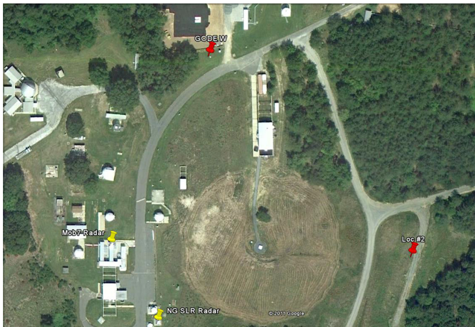
Figure 1: Geographic layout of GGAO outlining locations of the MOBLAS7 and NG SLR radars (yellow markers) as well as GODEW and Loc #2 points (red markers) where power reception measurements were taken.
