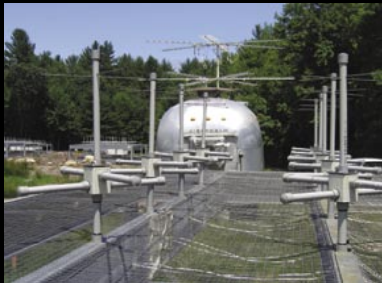
▲ Station with active crossed dipoles and beam directors. An RFI monitor system is shown in the background on the roof of the trailer.
