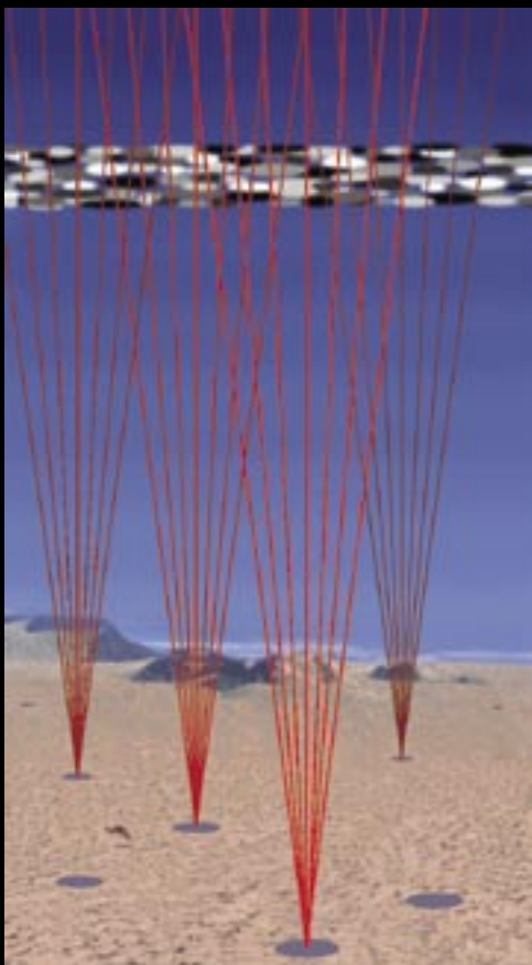
▲ The ray paths (in red) from individual MWA sub-arrays (grey disks) will overlap, permitting high-precision tomography of the ionosphere above the array.
