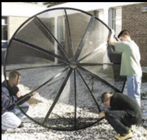
▲ Students from Shawsheen Valley Technical High School put together a Small Radio Telescope kit.
