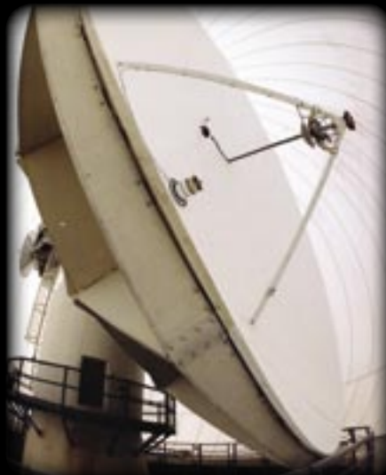
◀ The Westford 18-meter radio telescope (housed in an inflatable radome) operates with radiometers at frequencies of 2.8 and 8.4 GHz as part of the international VLBI geodetic network.
