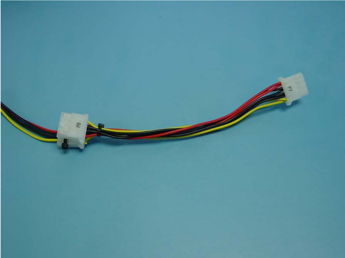
Figure 1: CD power cable
