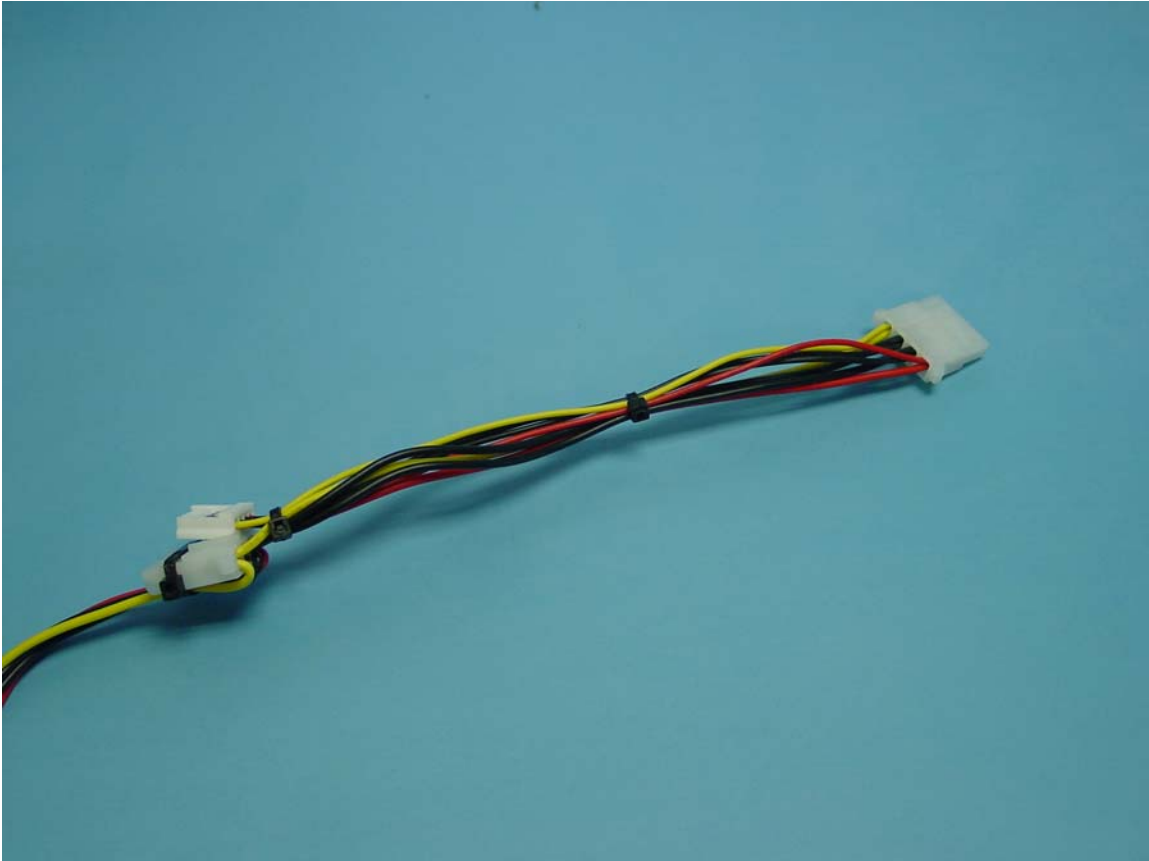
Figure 2: Hard Drive power cable
