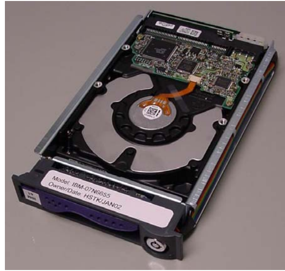
Figure 4: Example of labeled disc carrier (top and bottom)
